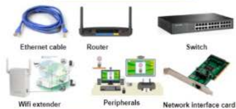
Typical hardware used to create a LAN.
